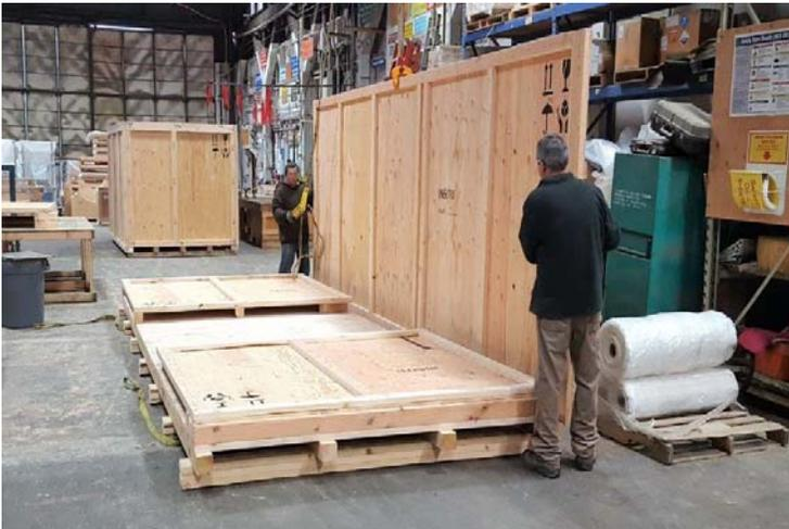
Base with two endwalls and one side wall
